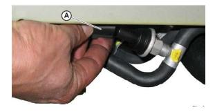
4. Unscrew and remove pressure sensor.
